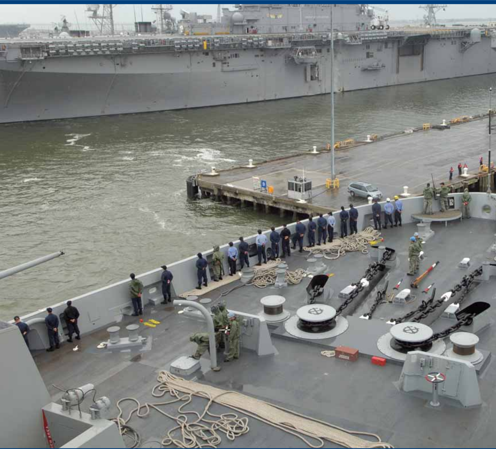
▲ Even the fo'c'sle of San Antonio has improvements, including a fresh water sprayer that washes the anchor chains as they are recovered to reduce corrosion.
