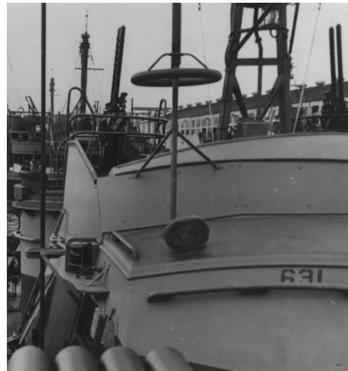
PT631 at factory shows IFF antenna in 1944
