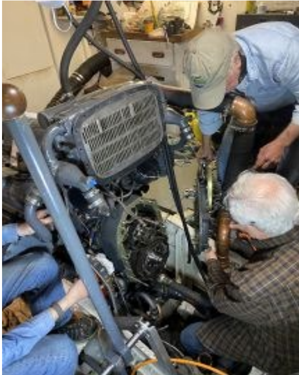
Left above: Volunteers removing the damaged supercharger drive shaft from the center engine. Right above: reinstallation of the impeller on the center engine following drive shaft replacement.
