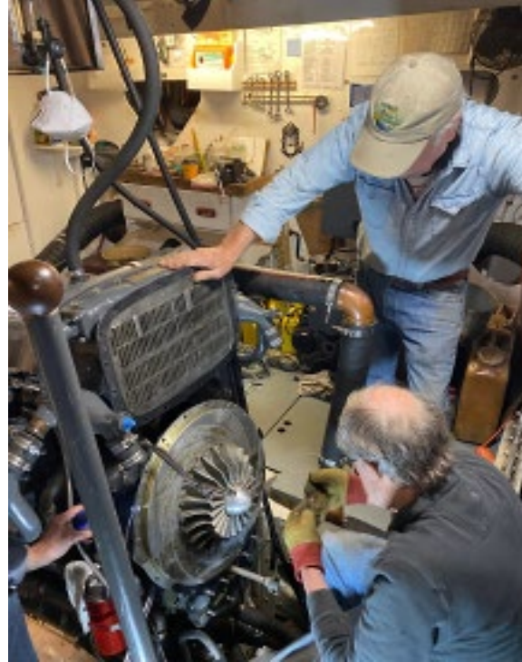
Left above: Volunteers removing the damaged supercharger drive shaft from the center engine. Right above: reinstallation of the impeller on the center engine following drive shaft replacement.
