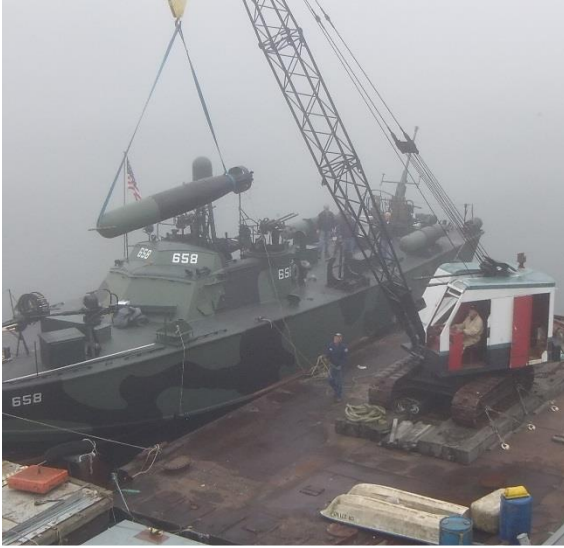
Above (L&R). Prior to drydocking, armament was offloaded to reduce weight and stress on the boat prior to lifting.
