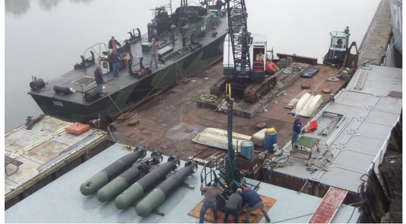
Below. On the day before the lift, the barge was towed to crane berth 312, along with the docking cradle stored on the barge deck. The docking cradle was lifted and lowered into the water by Vigor's 200 ton whirly crane. PT 658 was then carefully maneuvered above the submerged cradle--the cradle and boat were then lifted together out of the water. The load was carefully placed onto the barge and transported back to PT 658's boatshelter by Clark Caffall and his Tugboat, Christie. THANK YOU, VIGOR INDUSTRIES & CLARK CAFFALL!
