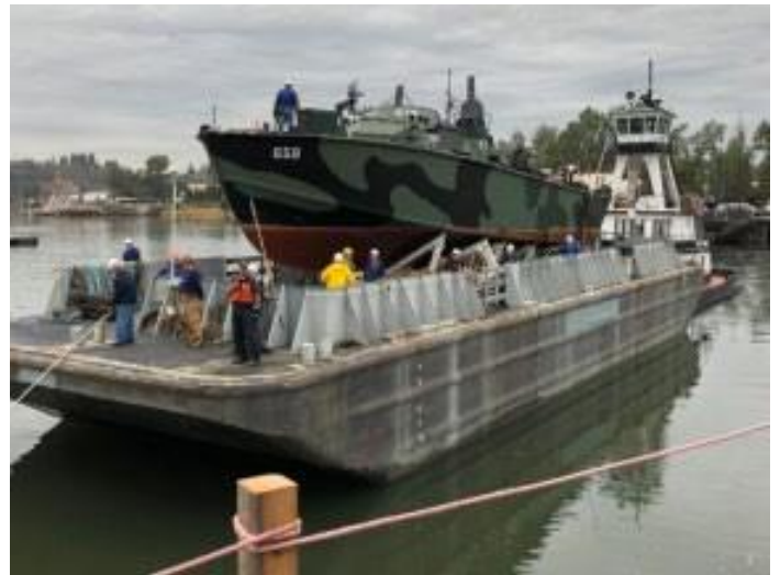
Below. On the day before the lift, the barge was towed to crane berth 312, along with the docking cradle stored on the barge deck. The docking cradle was lifted and lowered into the water by Vigor's 200 ton whirly crane. PT 658 was then carefully maneuvered above the submerged cradle--the cradle and boat were then lifted together out of the water. The load was carefully placed onto the barge and transported back to PT 658's boatshelter by Clark Caffall and his Tugboat, Christie. THANK YOU, VIGOR INDUSTRIES & CLARK CAFFALL!
