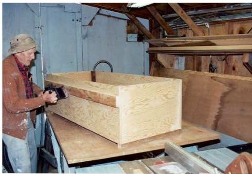
Bob Hostetter building the ammunition box for 40 mm. shells, similar to two others built for 20 mm. shells and installed just ahead of the charthouse on the bow.
