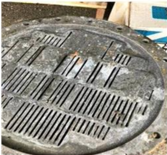
Unserviceable Heat Exchanger with Plugged Tubes, and Restored Heat Exchanger above
